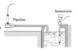
Pipeline Installation: Connect the 3/4" thread of the sensor head to the pipeline.
