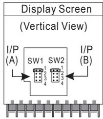
\*\*To Select the pin to modify the input signal for different sensors.
