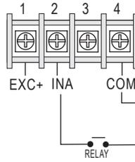
Relay Contact: NPN 0~400 Hz
