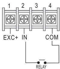
**Relay Contact: NPN 0~100 Hz**
