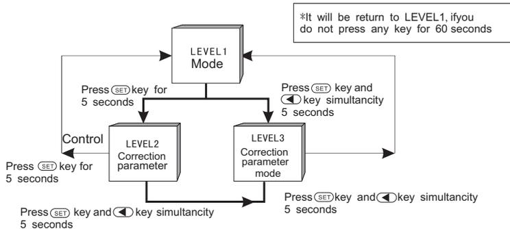
Press (SET) key and ◀ key simultancity 5 seconds
