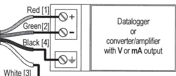
Connect to ground only if it is not possible to ground locally the case of the pyranometer
