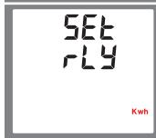
Press **E** to enter the selection routine. The unit symbol will flash. Use **M** and **P** buttons to choose kWh or kVArh.
