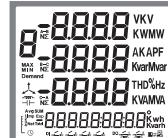
The first screen lights up all display segments and can be used as a display check.
