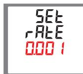
Press **E** to enter the selection routine. The current setting will flash. Use **M** and **P** buttons to choose pulse rate.
