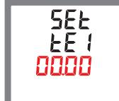
Press button **E** to enter set-up interface, there is the Period 1 start time information. The format is HH-MM. The left side picture show period 1 start from 00:00. Please press button **E** to activate the modification to change the time.
