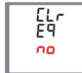
From the Set-up menu, use **M** and **P** buttons to select the reset option.
