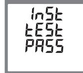
The interface performs a self-test and indicates the result if the test passes.
