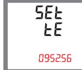
Press button **E** to enter set-up interface, there is the time information. The format is HH-MM-SS To change it , please press **E** button to activate the modification. The digits will flash. Use **M** and **P** buttons to choose the correct time information.
