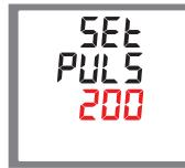
Press **E** to enter the selection routine. The current setting will flash. Use **M** and **P** buttons to choose pulse width(200/100/60ms)
